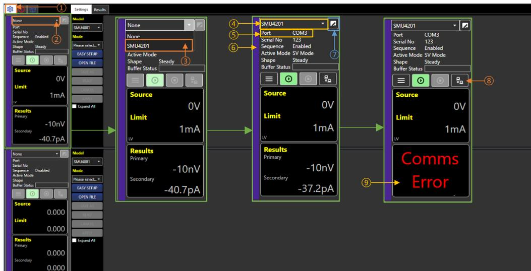
Select the drop-down box in the Instrument Control Panel ② to show all instruments available.
