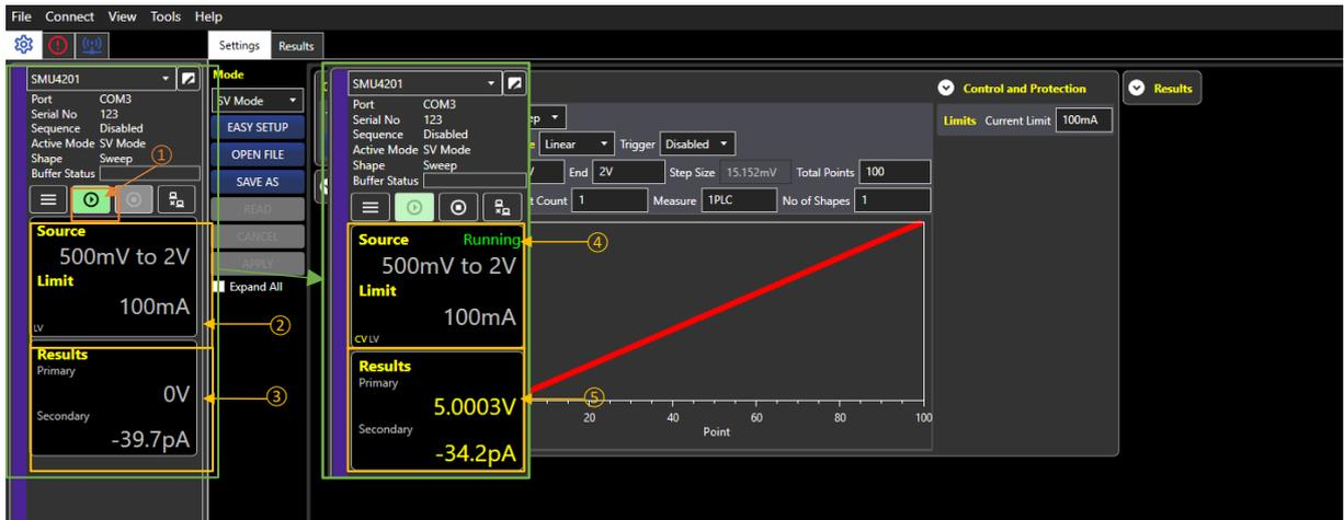
To run the setup, use the Run button ①.
