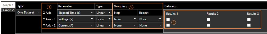
Allows the plotting of data from multiple datasets. Choose X and Y parameters, axis type (linear or log), and grouping ③. For each dataset, tick to show on the primary and/or secondary y-axis ④.
