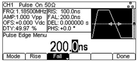
Alternatively the edge time can be entered as a percentage of the pulse width.
