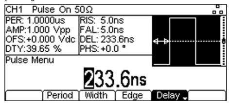
The Graph box shows the delay parameter between the arrows.
