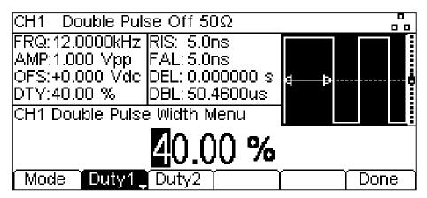
Setting up of Double Pulse is identical to setting Pulse parameters (as described earlier), but with the additional parameter of delay between the pulses.
