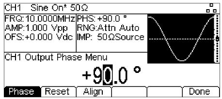
The convention adopted for the phase relationship between generators is that a positive phase setting advances the slave generator with respect to the master and a negative setting delays the slave generator. Phase changes on either generator will not cause a loss of synchronisation.
