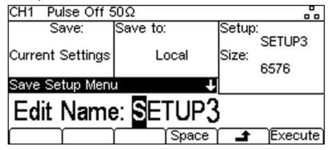
The current name can be changed if required. A name of up to 8 characters can be used. The cursor keys <> are used to select the character and the spin wheel used to change the character. When the wheel is turned clockwise the characters change in the following order: 0 to 9, A to Z,  $^{^{\prime}}$  (space)! # \$ % & ' () -
