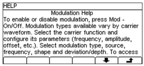
Below the topic heading is the topic text. If there is more text than will fit on the screen press the \$\ \ \\$ soft-key to scroll the text up one line. Continue scrolling until there is no more text indicated by the \$\ \ \\$ soft-key label disappearing.
