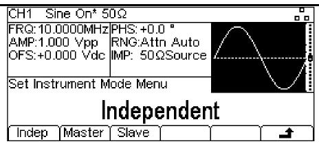
Press the **Master** soft-key to set the instrument as master. The signal at the MAIN OUT from the generator will stop at the dc offset level. Press Done.
