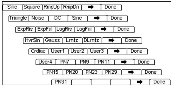
The large number of waveform shapes available include Arbitrary Waveforms and PRBS. See the sections describing Function/Arbitrary and Pattern/PRBS generator for details.
