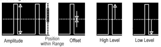
The maximum and minimum voltage levels depend upon the source and load impedances. The maximum and minimum EMF amplitudes (high impedance load) are 22V pk-pk and 200mV pk-pk respectively. The maximum and minimum high and low EMF levels are +11V and -11V.
