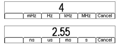
During the numeric data entry a decimal point and, if appropriate, a sign may be entered. The +/- key is used to alternately change the sign between + and -. The left cursor key may be used to erase the last digit entered. The entry may be cancelled by pressing the Cancel key
