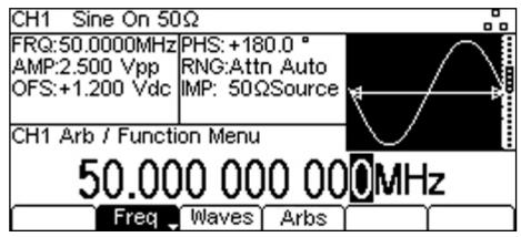
Parameters are set in terms of a Frequency (or Period) and a Waveform type. A further soft-key appears for certain waveform types including Square and Sinc.
