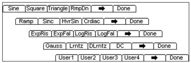
Pressing the **Done** soft-key selects the waveform and returns to the main waveform menu. A graphical representation of the waveform appears in the Graph Box.
