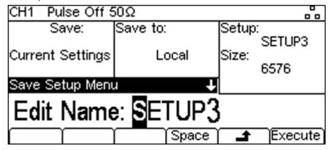
The current name can be changed if required. A name of up to 8 characters can be used. The cursor keys <> are used to select the character and the spin wheel used to change the character. When the wheel is turned clockwise the characters change in the following order: 0 to 9, A to Z,  $^-$  { }  $^-$  (space) ! # \$ % & '() -
