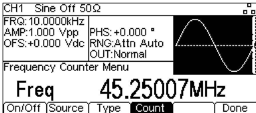
The Edit Box shows the current measurement. With no input signal at the selected input, the counter displays 'No signal' until an adequate input signal is applied.
