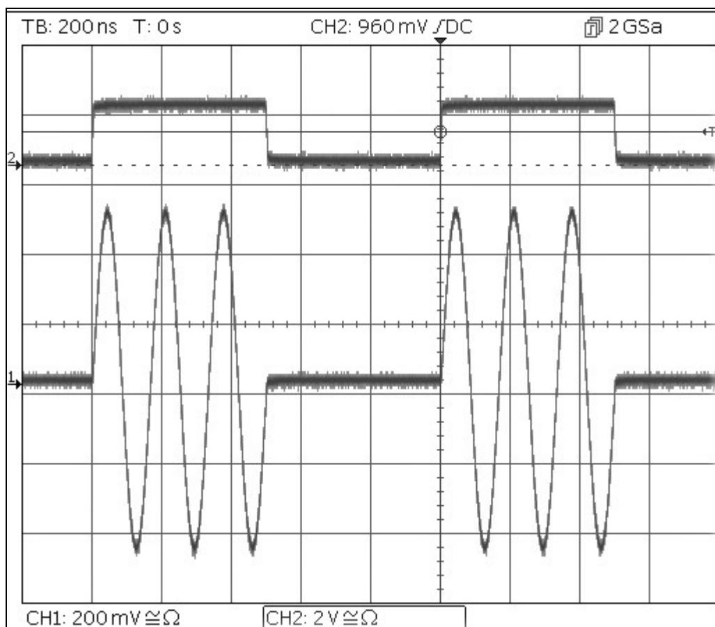
Note that the second trace is the output from the Main Output 2 socket when Channel 2 is synchronised which follows the trigger input signal.
