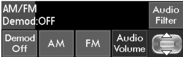
This menu controls the settings for demodulated audio in Zero Span mode, which can be Off, AM, or FM. The demodulated audio is outputted from the 3.5mm stereo/mono jack socket.
