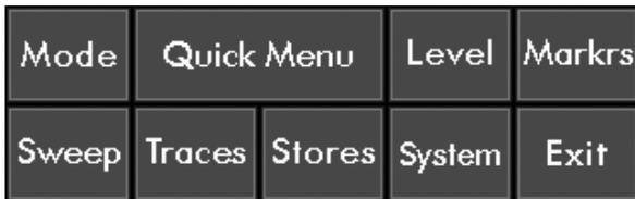
Quick Menu mode is selected using the Mode menu. Once selected, the two keys to the right of the Mode key change to become a single key marked Quick Menu.
