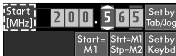
**The Menu Highlight Position:** When using the 5-way navigator for control, pressing the select button operates the currently highlighted key. On leaving a menu, this position is remembered and is recalled when the menu is next entered. Thus, if Start = M1 was the last function used within the Start menu, it can be operated again by highlighting Start in the Home menu and pressing the selector button twice.
