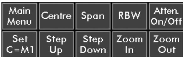
Selecting Quick Menu produces a new operating menu screen using dark green keys in place of blue. Operation using this menu is different from the other menus within PSAnalyzer.
