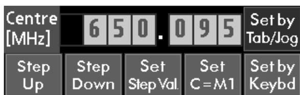
This menu allows the centre frequency of the sweep to be set. Values are always in MHz with a maximum resolution of 0.001 (1kHz). The range is 0.310 to 1299.840 MHz or 1.160 to 2699.840 MHz. The current centre frequency is displayed within the menu area.
