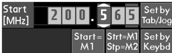
This menu allows the start frequency of the sweep to be set. Values are always in MHz with a maximum resolution of 0.001 (1kHz). The range is 0.150 to 1299.680 MHz or 1.000 to 2699.680 MHz. The current start frequency is displayed within the menu area.
