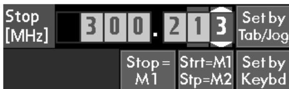
This menu allows the stop frequency of the sweep to be set. Values are always in MHz with a maximum resolution of 0.001 (1kHz). The range is 0.470 to 1300.000 MHz or 1.320 to 2700.000 MHz. The current stop frequency is displayed within the menu area.
