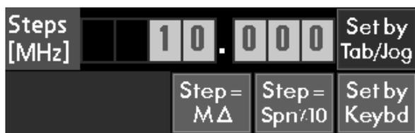
This is a sub-menu of the centre menu. It sets the step value that will be used in the Step Up/Step Down function of the centre frequency menu. Values are always in MHz with a maximum resolution of 0.001 (1kHz). The range is 0.001 MHz to 100.000 MHz. The current step value is displayed within the menu area.
