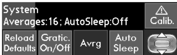
This menu is used to set the graticule display, set the averaging number for sweep averaging, and to set the delay time for auto sleep. The factory default set-up status can also be reloaded. The current status is shown within the menu area.
