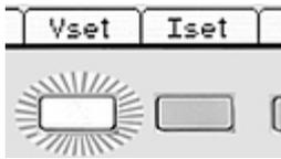
With the exception of output On/Off, the primary control of the power supply is via the six keys directly below the display. These are referred to as “soft keys” because their function is not fixed but is annotated by legends on the display directly above.
