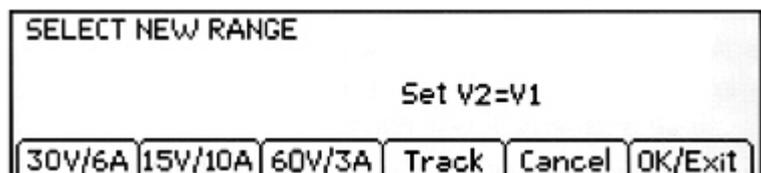
Voltage Tracking can be turned on or off from the Range menu of the output 2 screen. Alternatively it can be selected from the System Menu, see section 9.1.
