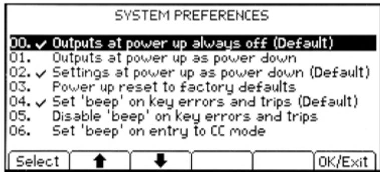
Changes are made by moving the highlight with either the arrow keys or the spin wheel and pressing the Select soft key.
