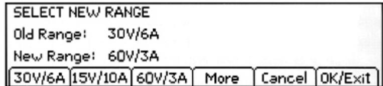
For output 1, the four additional ranges are selected by pressing the More key. For the 120V range only, a flashing HV lightning symbol will appear when a voltage above 60V is set.
