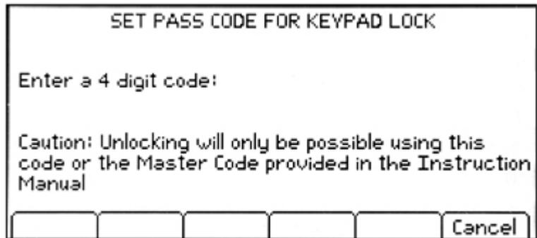
In the event that the user forgets the pass code, the power supply can be unlocked using the master pass code of 7835 which is always active.
