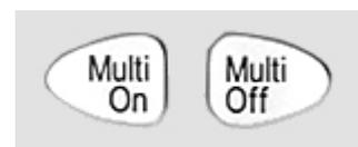
The System Menu function “Multi-On/Multi-Off Setup” enables the operation of these keys to be changed to suit the user’s requirements. Delays between the switching of the outputs can be introduced to create an On or Off sequence, and any individual output can be excluded from Multi-On or Multi-Off control.
