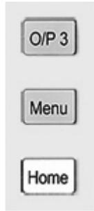
The function of the keys depends upon the type of screen selected. There are five main screens which are selected by the keys to the right of the display. The selected key is illuminated.
