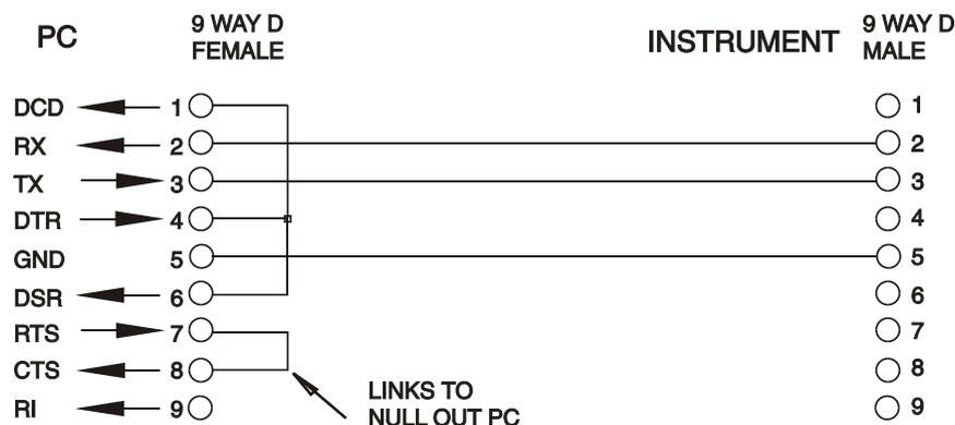
Most commercial cables provide these connections.
