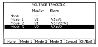
Three alternative voltage tracking arrangements are possible:
