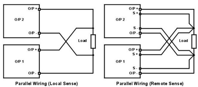
The drawing shows a parallel connection of two outputs using local or remote sensing.
