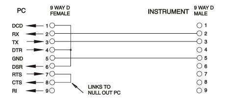
Most commercial cables provide these connections.
