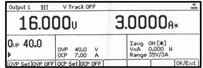
entered using the numeric keypad or by the spin wheel if enabled. OVP can be turned off by pressing OVP OFF, and turned back on by pressing OVP On. The previous OVP value is retained when OVP is off and is displayed in brackets.
