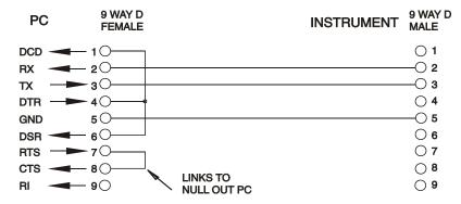
Most commercial cables provide these connections.
