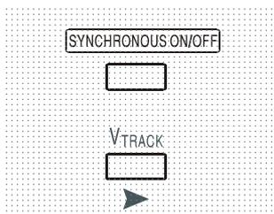
Pressing  $V_{TRACK}$  selects voltage tracking mode. The two outputs remain electrically isolated but the Voltage controls of Output 1 (the Master) set an identical voltage on Output 2 (the Slave).
