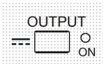
At power on, the factory default setting is for the output to be off. The preset output volts and current will be determined by the present control settings and shown in the display. The VIEW lamp is lit to indicate that it is the preset values that are being displayed. All other settings will be the same as they were at last power off.
