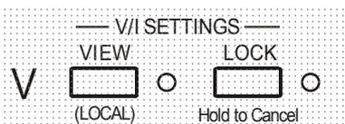
If the output is still on, **OP on** (output on) will flash twice in the display, followed by flashing of the new 'unlocked' settings for 2-3 seconds (slowly at first, then faster) before the change is finally implemented; the LOCK lamp goes off when the change is made.
