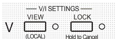
The set voltage and current limit are always shown when the output is off but can also be viewed when the output is on by pressing the VIEW key; the VIEW lamp is lit whilst the VIEW key is pressed.
