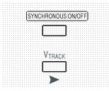
Pressing  $V_{\text{TRACK}}$  selects voltage tracking mode. The two outputs remain electrically isolated but the Voltage controls of Output 1 (the Master) set an identical voltage on Output 2 (the Slave).
