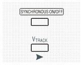
The SYNCHRONOUS ON/OFF key is in addition to the individual OUTPUT switches and permit both outputs to be turned on or off synchronously with a single key press. Since this key turns both outputs on or off with alternate presses it is necessary for both outputs to be in the same state (i.e. both on or both off) before the key is used. Pressing the key with one output on and one output off will have no effect.
