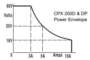
The power envelope is set to give 60V/3A, 35V/5A and 16V/10A under all supply conditions (both outputs loaded); at lower output voltages the output power is restricted by the 10A current maximum.
