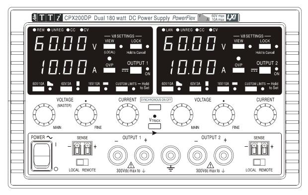
The load should be connected to the positive (red) and negative (black) terminals marked OUTPUT. The OUTPUT terminals are rated at 30A.
