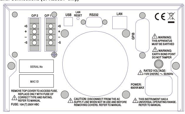
The output and sense terminals for OUTPUT1 and OUTPUT2 are duplicated on the rear panel terminal blocks and are marked +, -, +S and -S. These connections are paralleled with their front panel equivalents.
