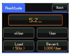
When on the editing screen, the digits can be entered directly from the keyboard in any convenient units, e.g. 12.34kHz can be entered directly in kHz but can also be entered as 12340Hz or 0.01234MHz, press the Hz or kHz unit entry buttons to set units and confirm entry.
