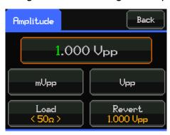
Select the editable field using the knob, press to enter the active editing state. Alternatively, jump straight to the editing state by touching the editable field.
