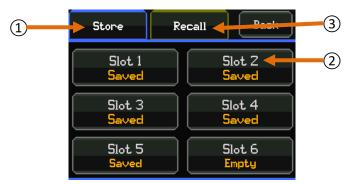
6 memory slots are provided, allowing the user to store and recall the settings for the instrument.
