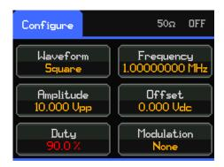
When using Sweep or FSK, if either of the set frequency values in combination with the duty value are out of the specified limit, the duty will be shown in red to indicate that the resulting waveform no longer meets specification and may not be as expected. See *'Technical Specifications'* for more details.
