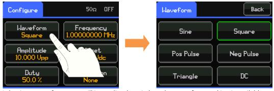
Selecting a waveform type will immediately switch to that waveform making it available at the MAIN OUT connector if the output is on, if the output is not on press the OUTPUT key to turn output on.
