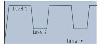
Slew rate control applies to all changes of level including remote control and manual changes between level A and level B.
