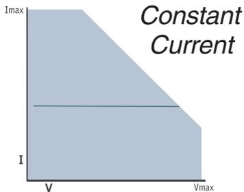
Constant current mode is used for load testing of normal voltage-source power supplies and for constant current discharge testing of batteries.
