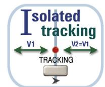
The two outputs of the CPX are completely independent and electrically isolated from each other. With V-Track selected, the two outputs remain electrically isolated, but the voltage control of the Master output sets an identical voltage on the Slave output.
