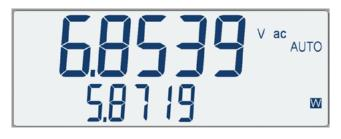
The VA function makes use of the dual measurement capability and displays the product of voltage and current.
