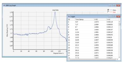
The application also provides a means of downloading the contents of the internal logger of the meter itself, and exporting it to a CSV file.
