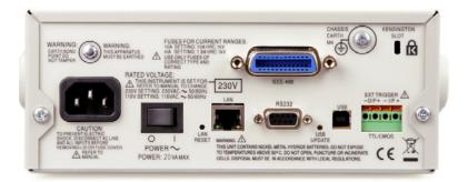
1908 rear panel (Protective buffer removed) GPIB optional.
