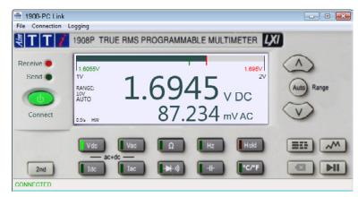
The application provides remote access to the instrument using a pointand-click interface arranged similarly to the actual instrument.
