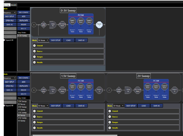
Figure 12- Aim-TTi Test Bridge SMU sequence setup.
