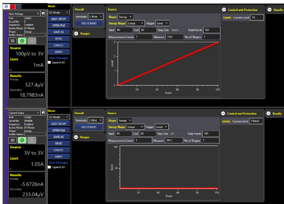
Figure 11- Aim-TTi Test Bridge SMU setup.
