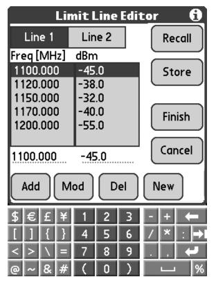
Limit lines are created by defining a list of frequency & amplitude points (minimum 2). Straight lines are drawn between these points. Where a frequency is repeated with different amplitudes, the line becomes vertical representing a step change.
