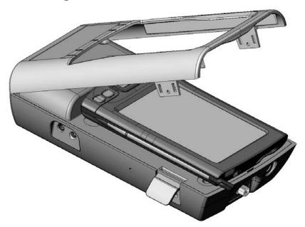
Lift the two latches close to the top of the unit and remove the silver top cover (see drawing). Remove the Palm T|X by gripping its sides and pulling it towards the top edge of the spectrum analyzer. (Note that the connector is a tight fit and that a hard pull may be needed).
