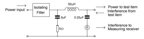
The defined impedance is provided by the 50 $\Omega$  input impedance of the measuring receiver in parallel with the series combination of the 50 $\mu$ H inductor and the 5 $\Omega$  resistor. These values define the variation of input impedance with frequency which is required by CISPR 16 and shown on page 17 of this manual.
