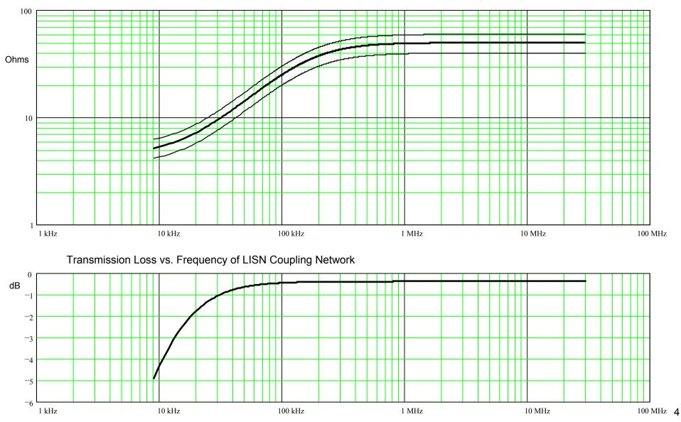
Input Impedance vs. Frequency of  $50\Omega \parallel (50\mu H + 5\Omega)$  CISPR 16 Network, showing nominal value and ±20% limits
