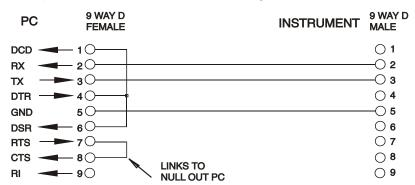
Most commercial cables provide these connections.
