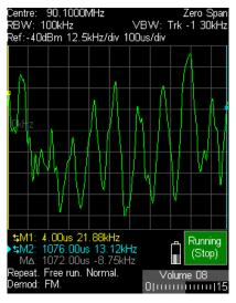
In addition to audio demodulation of AM or FM signals, the modulating waveform can be displayed against a timebase settable between 5us/div and 20ms/div. Markers can be used to
