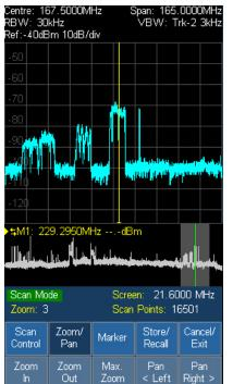
Scan Mode is an entirely different mode of operation in which a narrow RBW can be set resulting in a much higher number of data points being collected - up to 210,000 points.
