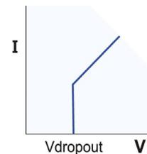
Resistive discharge (conductance mode) with voltage dropout.
