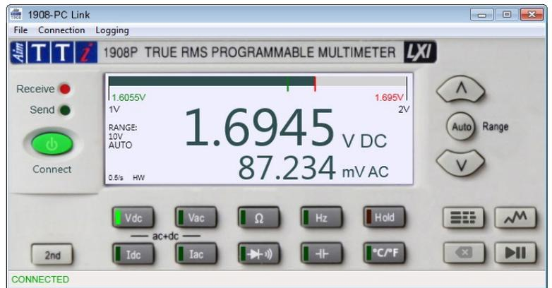
The application provides remote access to the instrument using a point-and-click interface arranged similarly to the actual instrument. Measurement function can be selected for both the main and secondary displays, along with measurement range. The display includes an analog bar-graph with minimum and maximum reading markers.
