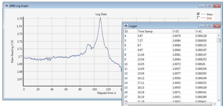
The application also provides a means of downloading the contents of the internal logger of the meter itself, and exporting it to a CSV file.
